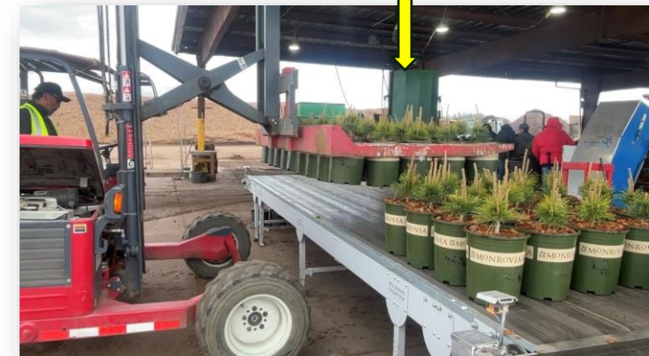
Widebelts at canning allow for continuous production, 12% improvement across the nurseries
