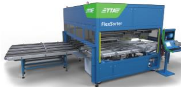
TTA Flex sorter: 3,000 to 12,000 plugs per hour
