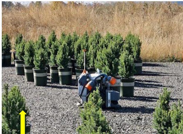
Spacing Robot: 200-250 plants per hour
